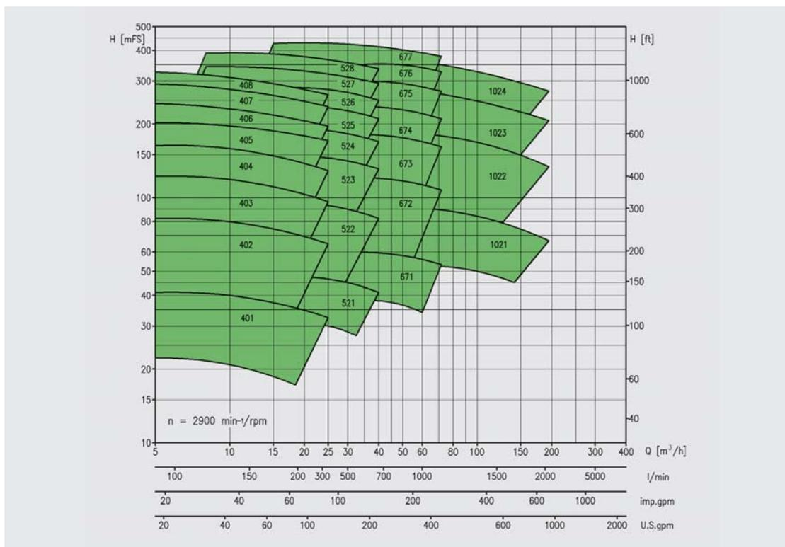
Performance curves for the individual pump sizes, also for 1750 / 3500 rpm, with NPSH-values and power consumption, are available on request.
