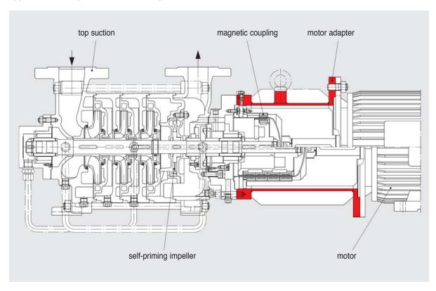
Type HZSMR – top suction with oil lubricated bearing bracket
