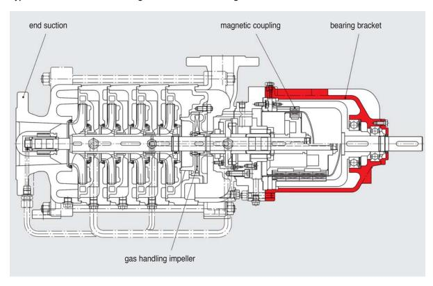
Type HZSMAR – end suction with oil lubricated bearing bracket
