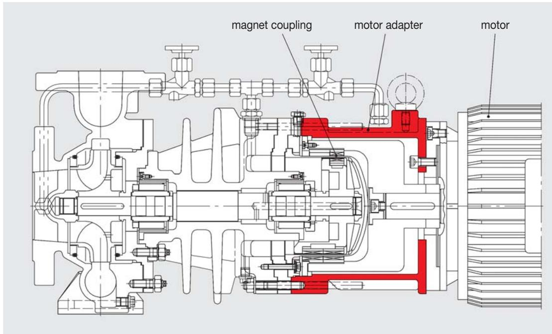
**Type NMW - with grease lubricated ball bearings**
